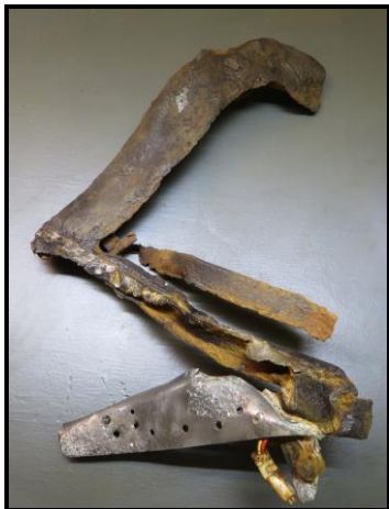
part of the cockpit structure of the Me-109
